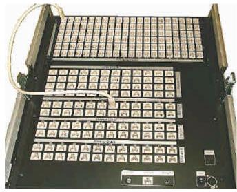
A Series patch requires two loads to be connected to work, this as the 2 loads will be wired in series with each other to allow the use of 110V lamps. The first bay allows two sets of loads to connected (thus four loads are needed)
